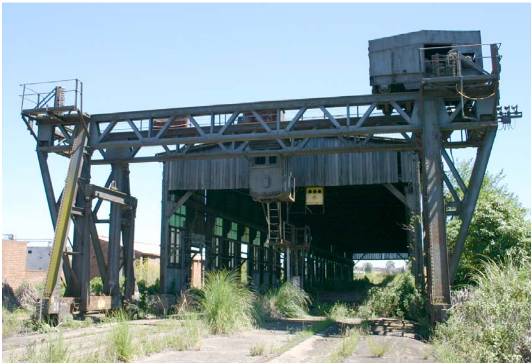
Figure 41. Mid-20th century electric-powered gantry crane outside of the Transhipment shed & wagon repair workshop. January 2005
