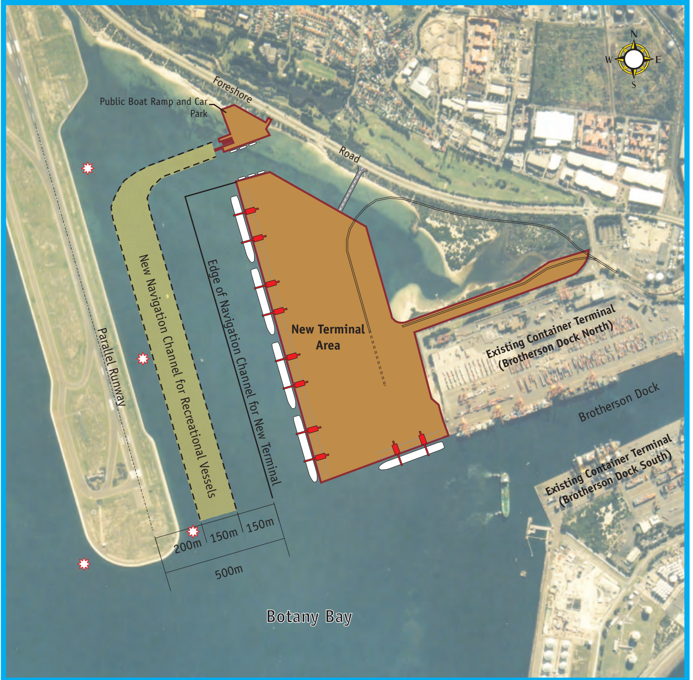
Navigation Channels at the New Terminal
