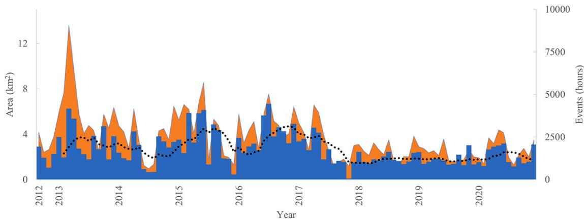
Fig. 3. Estimates of hours (orange) at anchor and area ( $\text{km}^2$ ) (blue) affected directly by anchor scour for the Port Kembla anchoring roadstead from Oct 2012 to Dec 2020. Dotted line represents a 6-month moving average of area anchored.
