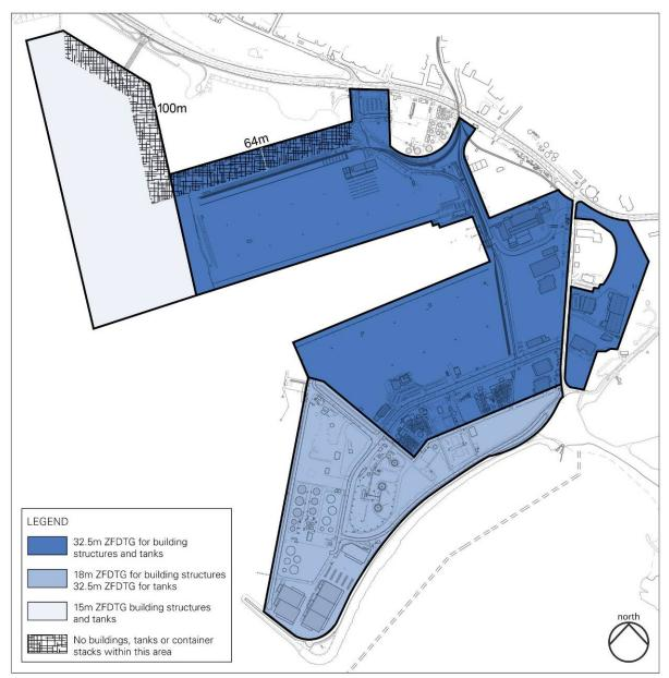
**Figure 1** – Maximum heights for building structures and tanks (Zero Fort Denison Tide Gauge (ZFDTG))
