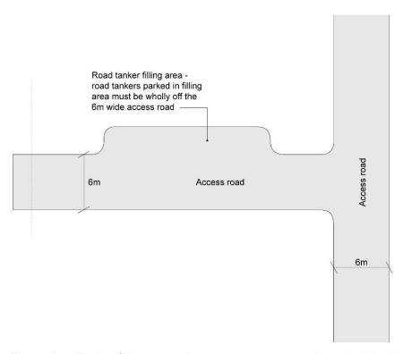
Figure 14 - Tanker filling area adjacent to an access road at a bulk liquid storage facility
