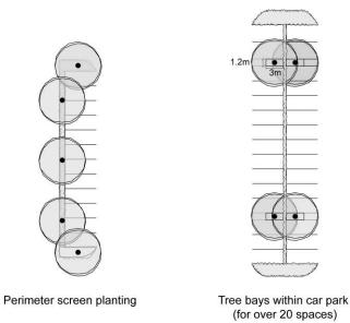
Figure 5 – Required perimeter screen planting (left) and tree bays within car parking areas (right)
