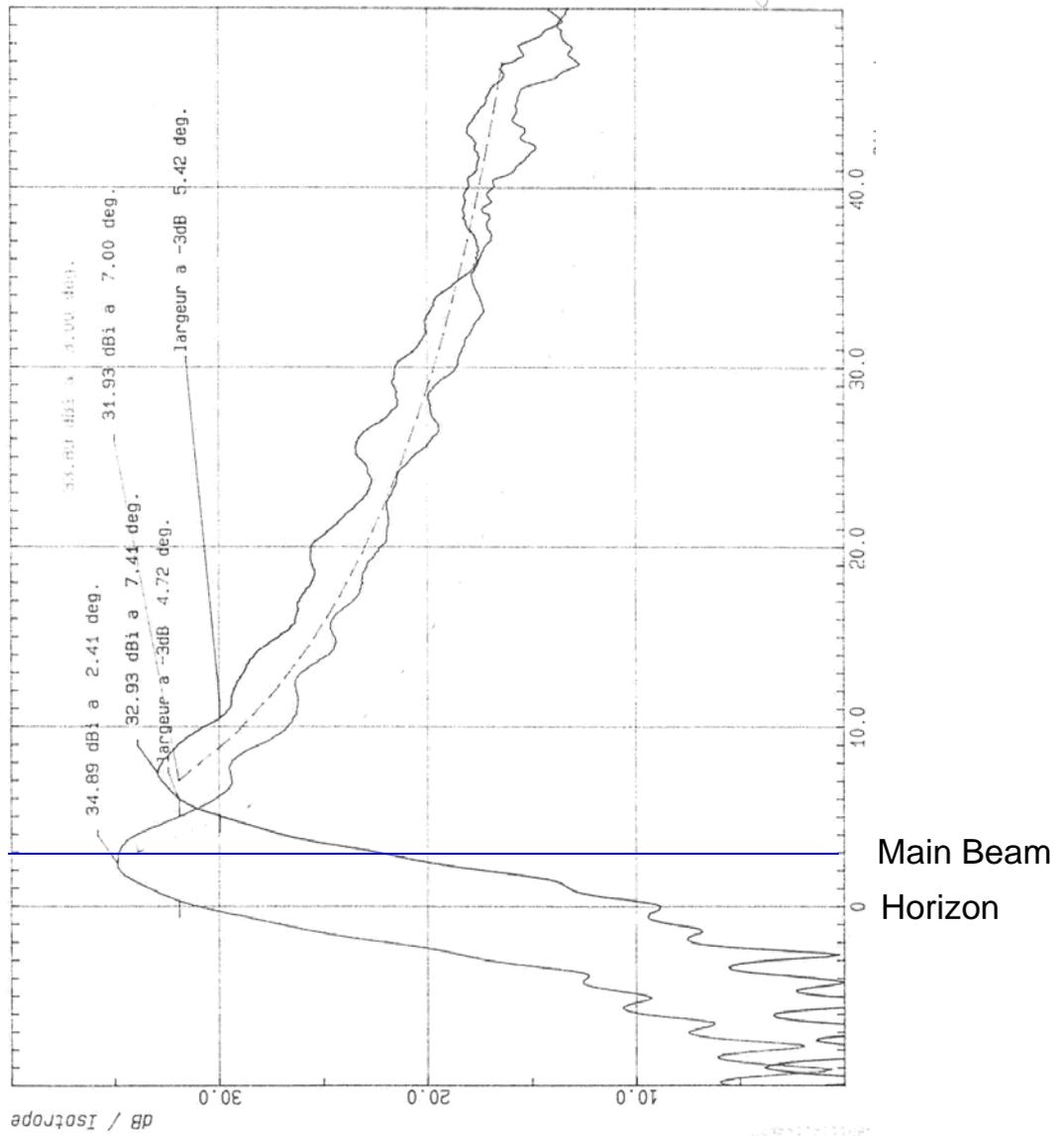
Figure 5 Tar Horizontal Radiation Pattern (Primary)
