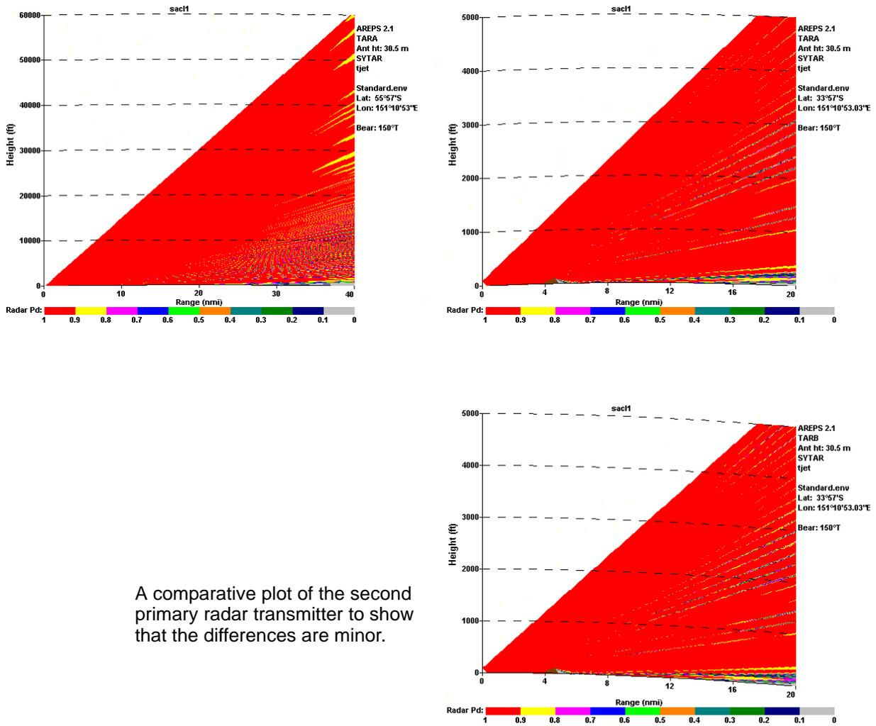
A comparative plot of the second primary radar transmitter to show that the differences are minor.
