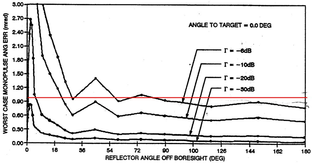
Figure C-3. Monopulse Angle Error Due to Horizontal Multipath
